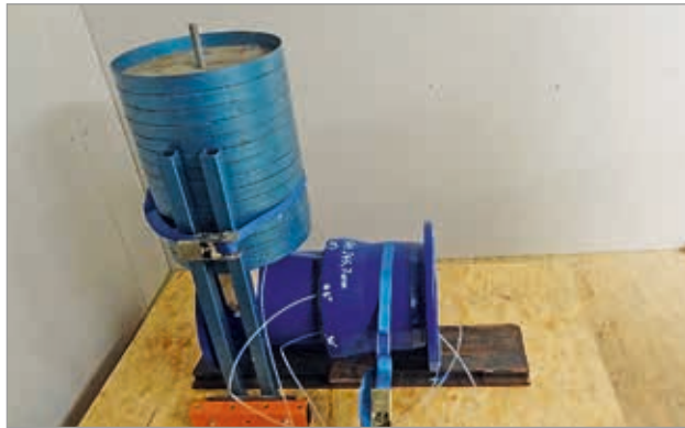
Test set-up for the TYTON® push-in joint
